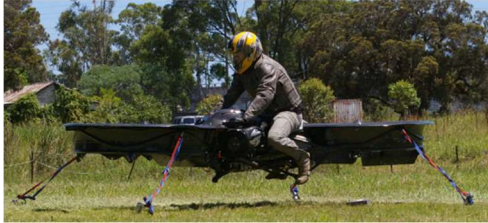
Figure 4 - Full scale pilot test [2]
